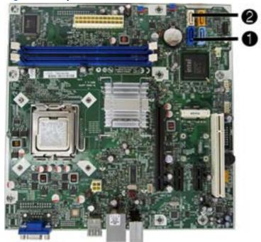
Figure 2-25 System Board Drive Connections — 500B/510B
